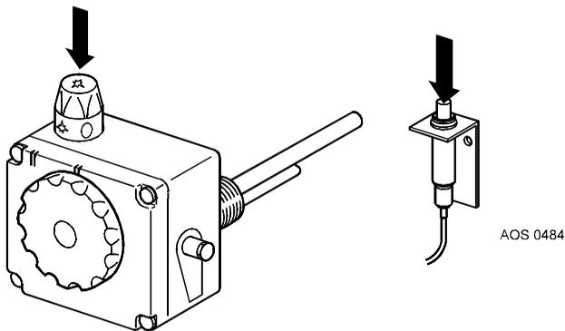
Drawing 6 - Operation of the gas control block
