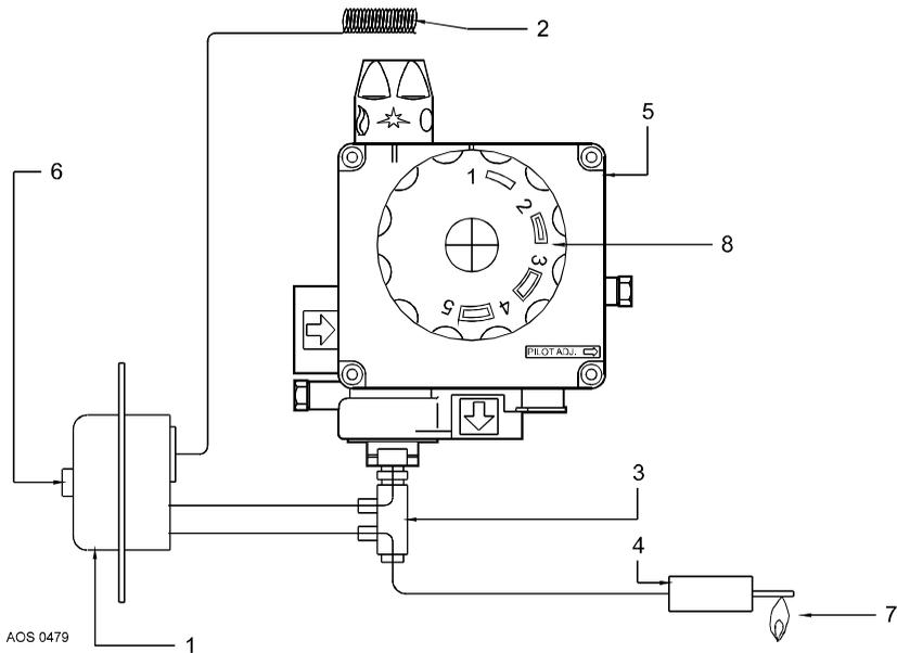
Drawing 2 - Gas control block with T.R.S.
