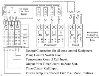
Under no circumstances should high and low voltage circuits be conducted through contacts on the same relay, as this would not comply with the clearances (minimum distance between switching contacts) specified by IE and international wiring regulations. If a control is required on a circuit of different voltage to the primary circuit, the auxiliary relay or a separate external relay should be used.
