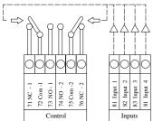
The Auxiliary relay is an optional control opportunity that works independently of the boiler control relay. Applying mains to any auxiliary input (81, 82, 83, or 84) will operate the double pole auxiliary relay contacts but will not back feed to other auxiliary inputs.
